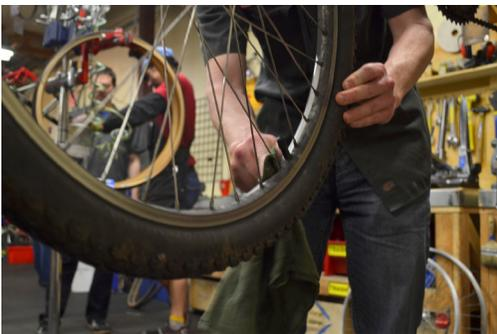
3. If they're really dirty (your silver rim looks uniformly black) start here, otherwise skip to step 4. Spray the rim with your cleaner of choice, scrub the top surface with an old toothbrush, and braking surface with a Scotch-Brite pad. Once all that grime is loosened up, wipe the rim with the clean rag.
