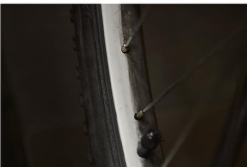
5. While you're wiping take a close look at the rim and brake pads. Make note of the rim profile; does it feel flat or concave? Look closely at the spoke/rim interface; do you see any tiny cracks? How do the brake pads look? Can you still see the grooves in the pad? If the rim feels concave, looks cracked, or the brake pads have worn past their grooves, something could be worn and should be looked at by a mechanic.
