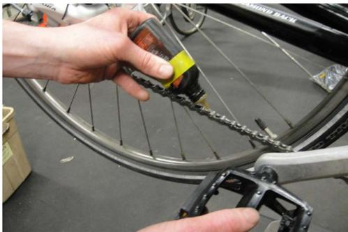
3. Now you're ready for oil. Pick something that's designed for bike chains, such as TriFlow or Phil Wood's Bio Lube, and avoid products like WD40, 3 in 1 oils, heavy grease, or anything in a spray can.
